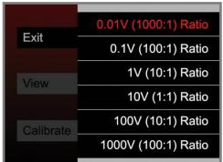
voltage reference, is used for the self-calibration of the voltage ratios. If a customer chooses, the 7520 also allows for an external null detector to be used to automatically calibrate the 7520 voltage ratios.
