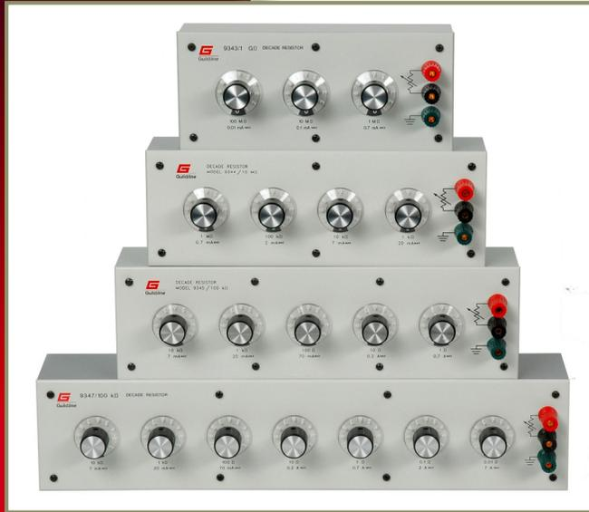
**GUILDLINE INSTRUMENTS 9340 SERIES** of precision DC Resistance Standards are a complete family of easy to use resistance standards offering the best combination of highest accuracy and widest range commercially available.
