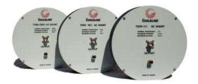
The 7350 Series of four-terminal AC Current Shunts are designed to be a lower uncertainty and more stable replacement of the successful Guildline 7320 series. These patented shunts also have a non-inductive design and are essentially purely resistive. With a ruggedized and shielded enclosure, the 7350 series shunts are constructed with very small values of reactance.
