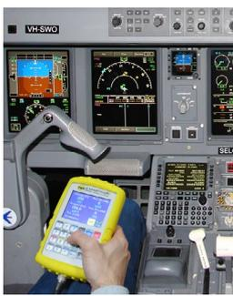
Optional MPSRC Hand held remote control unit: Multi-coloured backlit 3.5" LCD touchscreen and keypad
