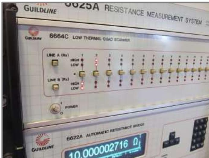
**THE 6664C LOW THERMAL QUAD CHANNEL SCANNERS ENABLES SOFTWARE CONTROLLED, FULLY AUTOMATED NORMAL AND HIGH OHM MEASUREMENTS WITH VOLTAGES UP TO 1000 V!**
