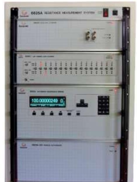
6625-300 Ampere System, from 1  $\mu\Omega$  to 1G $\Omega$  with single 6664C Scanner
